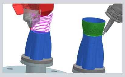
Hybrid manufacturing unifies additive and subtractive operations, enabling production of next-generation designs with tight tolerances.
