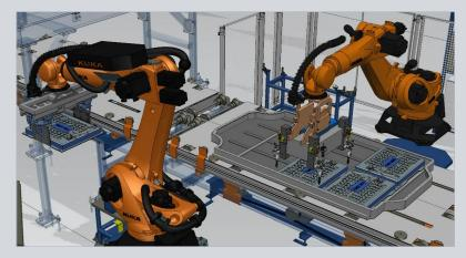
Advanced robotic simulation with automated motion planning reduces the most time-consuming tasks in programming by up to 80 percent.
