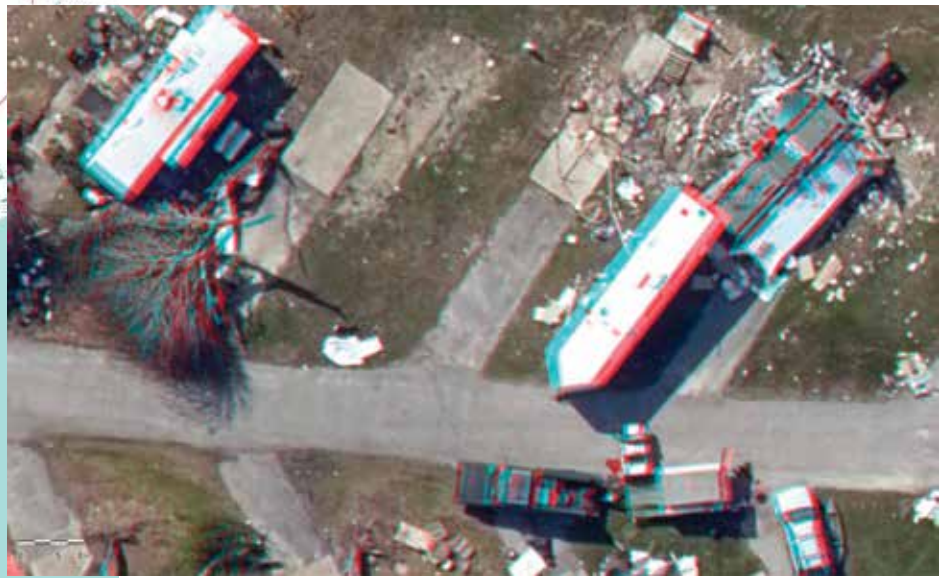
↑ With stereo orthoimagery, which is viewed with 3D glasses, users got a better idea of where the storm knocked down trees or winds ripped the roofs off houses. (Imagery courtesy of Vexcel Imaging.)
